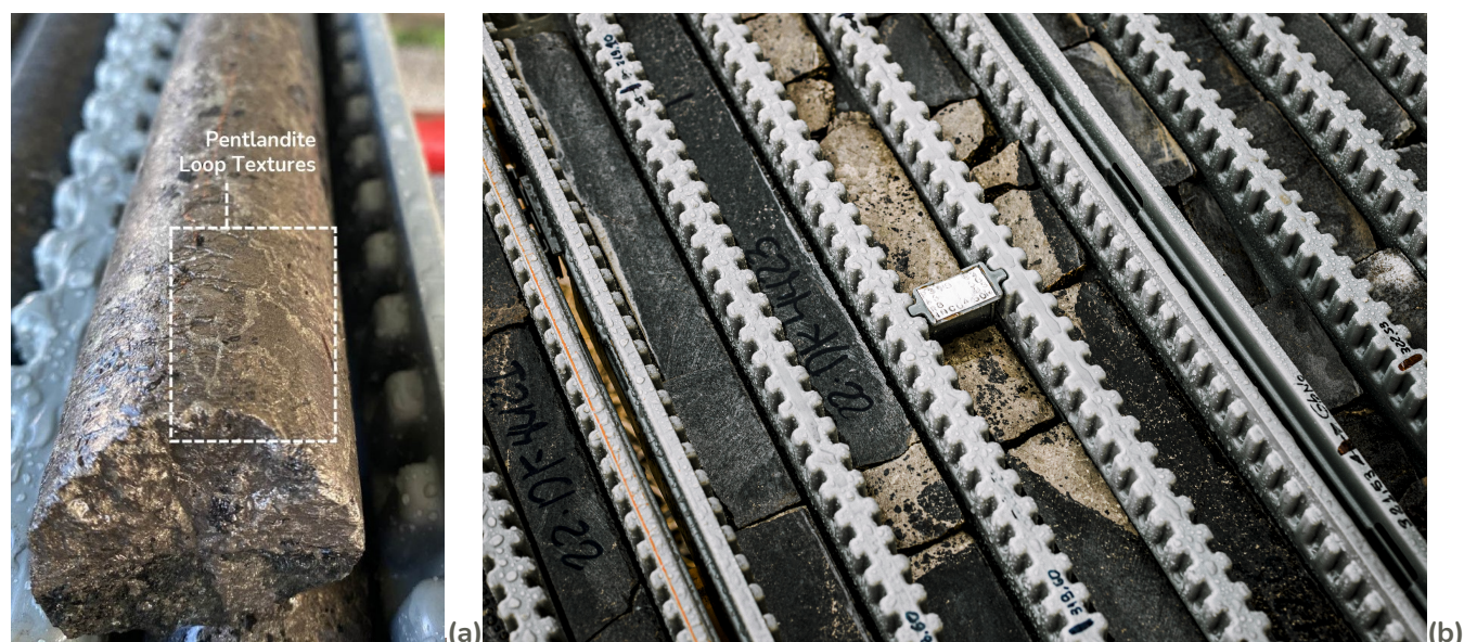
Figure 1: Drill core from the deepest intercept to date in the VB Zone (hole VB-25 at ~319 meters) highlighting loop textured pentlandite in (a) and high-grade massive sulphide intervals within the zone (b).
