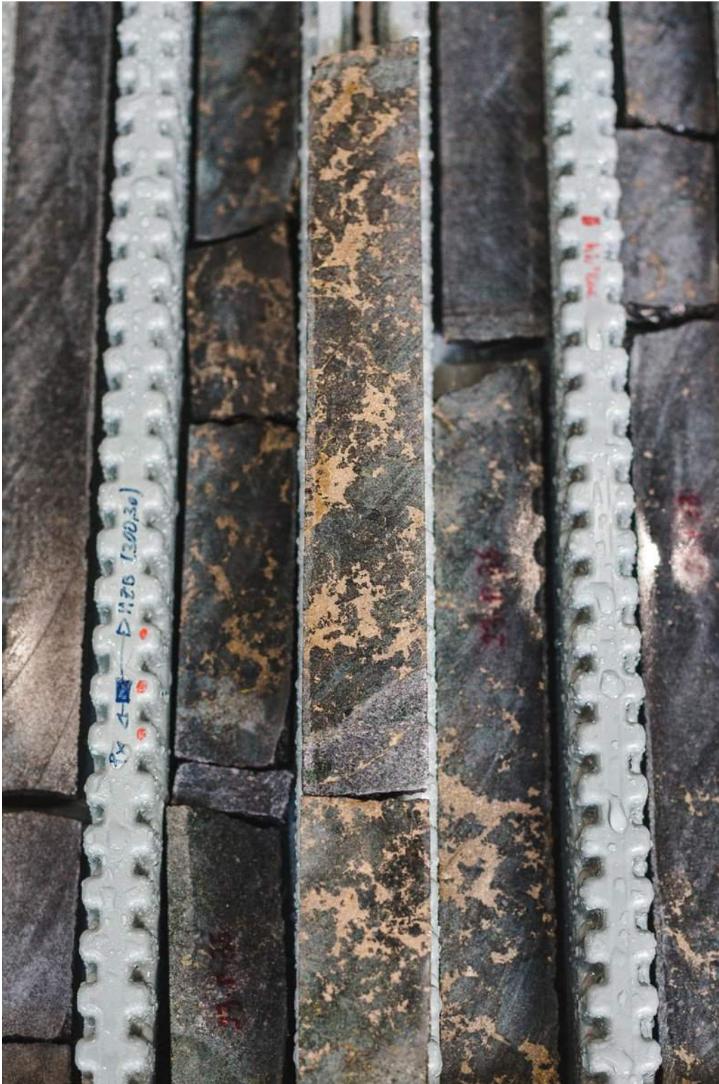
Figure 4: Brecciated and patchy net-textured sulphides shown in detail for hole LZ-32 (~300 meters downhole) showing both pentlandite and pyrrhotite
